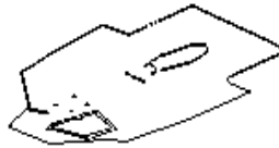
No 31. 964/993 forward tunnel section
